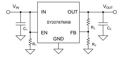
Figure 1. Adjustable Output Regulator
