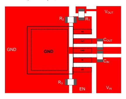
Figure 3. PCB Layout Suggestion
