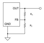
Choose R2 and R3 to program the proper output voltage. Choosing large resistance values for both R2 and R3 is recommended to minimize power consumption under light loads. A value of between  $10k\Omega$  and  $1M\Omega$  is recommended for both resistors.
