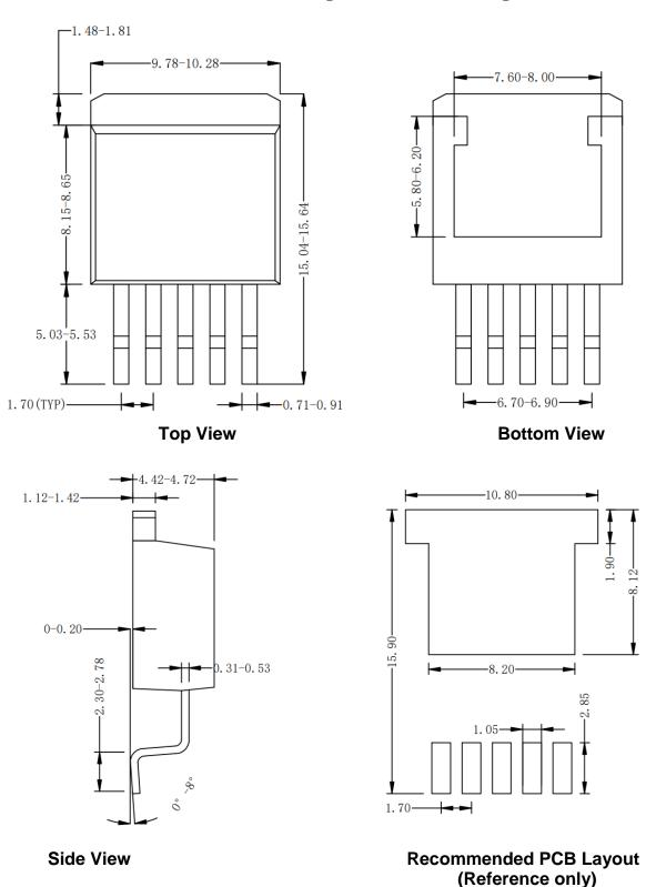
Note: All dimensions are in millimeters and exclude mold flash and metal burr.
